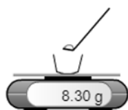
Measuring out 8.30g of potassium iodide powder with a digital balance (accurate to 0.01g).
