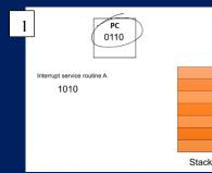
The PC holds the next instruction address. Interrupt service routine A needs to be ran. The value of the PC is stored in the stack until the ISR has been completed. The value in the stack is then moved back into the PC so the CPU knows where to begin processing from again.
