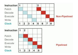
We can see on the left how the non-pipelined CPU took more clock cycles and so longer to complete the two instructions as making efficient use of its resources (some of the stages are idle and should be used).
