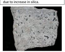
Trachyte Fine grained light white coloured hypabyssal or extrusive rock. Has an aphanitic and porphyritic texture. Phenocrysts of orthoclase. Grey with white crystals
