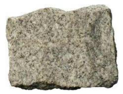
Microgranodiorite Medium grained intermediate rock with increasing quartz. Formed of mainly plagioclase than orthoclase. Light appearance.
