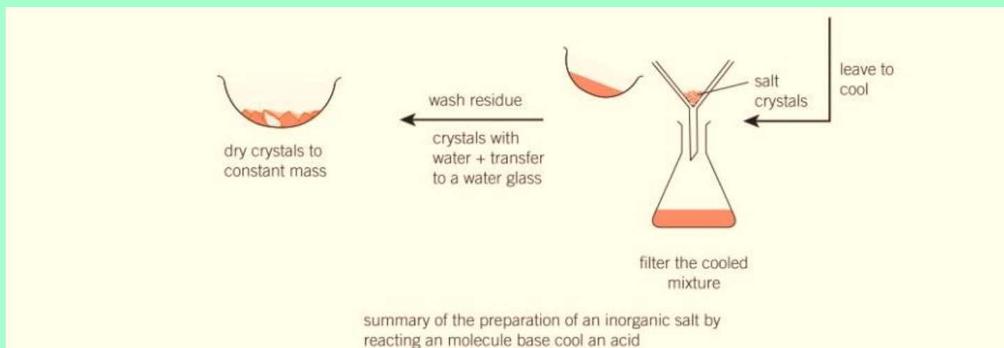
▲ Figure 7 Summary of the preparation of an inorganic salt by reaction of an insoluble base with an acid
