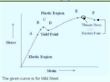
Like many metals, there is an elastic region to begin with (O to B). Any stress here results in elastic deformation, once the stress or force is removed the original strain or length/shape is resumed.
