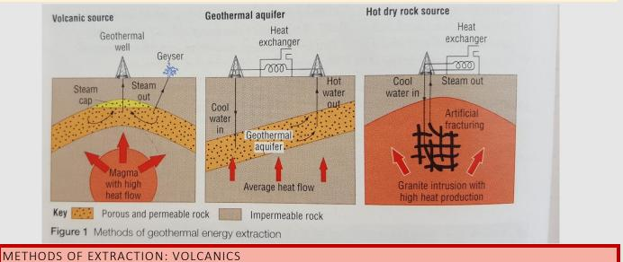
In volcanic areas, magma at **temperatures of 700<sup>o</sup>C to 1000<sup>o</sup>C** heats the **gr**oundwater contained within surrounding rocks/ an aquifer.
